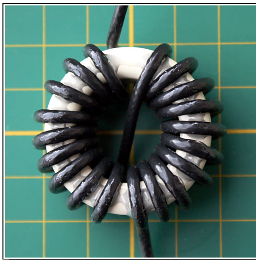
Traditional low-capacitance construction with split winding.
